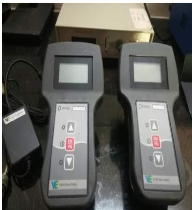
DIGITAL H 2 S AND CH 4 ANALYZER
